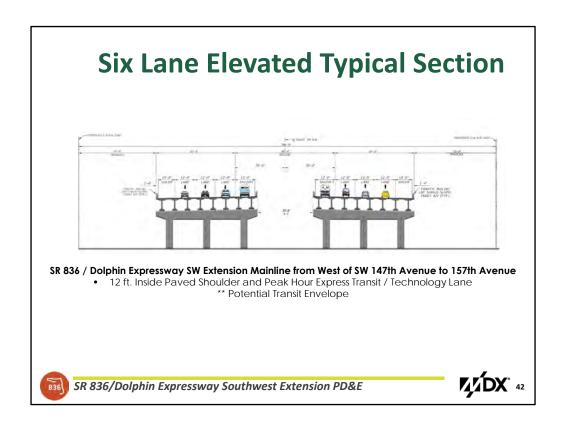
An elevated typical section was considered in sensitive areas as appropriate. The segment along SW 8th Street (Tamiami Trail) is mostly elevated as shown here to avoid or minimize impacts to sensitive lands.
