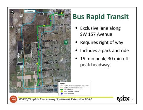
In this alternative, a Bus Rapid Transit or BRT alternative along SW 157 was evaluated assuming additional right of way would be purchased to accommodate BRT in an exclusive lane and assuming the facility would be constructed and operated by others
