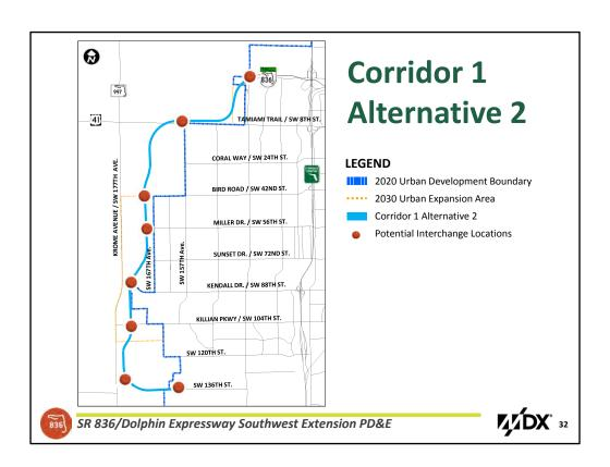
Alternative 2 includes 7 proposed interchanges. In addition to the interchanges proposed for Alternative 1, Alternative 2 includes two additional interchanges: are at Miller Drive and the other at Killian Parkway
