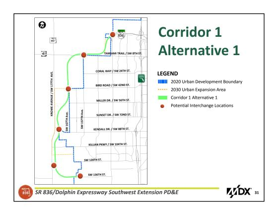
Both alternatives for Corridor 1 generally follow a more westerly alignment. Alternative 1 includes 5 potential interchanges which includes the expansion of the existing interchange at NW 137<sup>th</sup> Avenue to include southbound and northbound access to and from NW 6<sup>th</sup> Street. Interchanges are also proposed at SW 8<sup>th</sup> Street with SW 157<sup>th</sup> Avenue, Bird Road and Kendall Drive as well as a direct connection to and from Krome Avenue.
