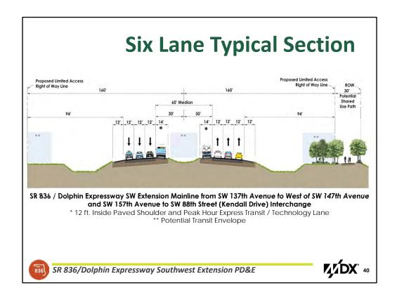
The proposed typical section consist of three lanes in each direction from the existing terminus of SR 836 to SW 88th Street (Kendall Drive)
