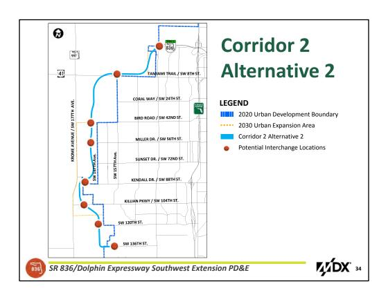
Alternative 2 proposes interchanges in the same locations as Alternative 1 while shifting the alignment near SW 167<sup>th</sup> Avenue slightly west to provide greater separation to existing homes while still remaining outside of the 10-day contour for the Wellfield to be described in further detail later in the presentation.
